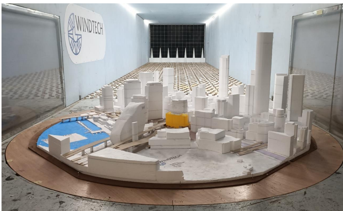
Figure 1e: Photograph of the Wind Tunnel Model (Proposed Scenario, view from the south-west)
