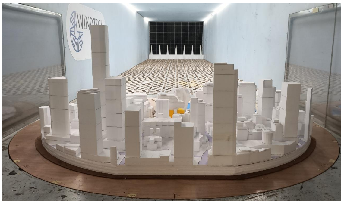
Figure 1c: Photograph of the Wind Tunnel Model (Proposed Scenario, view from the east)
